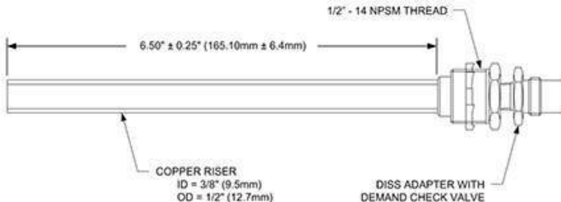
Figure 10. Stryker-supplied Gas Riser with Check Valve
